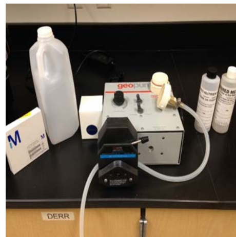
Figure 6 Filtering chemistry samples using a GeoPump
