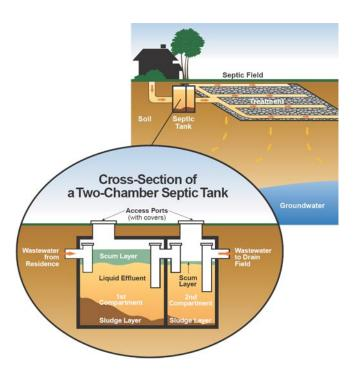
Through bacterial action, some of the solids are digested and converted to liquid for discharge into a "soil absorption area" or leach field. The remaining solids are stored for future disposal.
