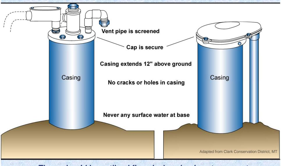
There should be antibackflow devices in place to prevent the flow of contaminated fluids into the ground water. Keep good records of all well inspections, repairs and water testing.
