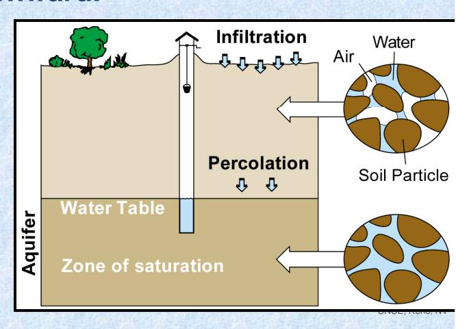
Underground deposits of water in this saturated zone are called aquifers.
