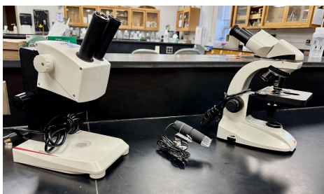
Figure 1. (from left to right) Standard Dissection Microscope, Digital Microscope, and Compound Microscope Photo: Kaitlin Campbell
