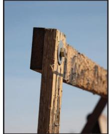
A single bolt screwed into a tnut securing the uprights to the crossbar allows you to fold them together if you ever want to pack it up and move it. For the same reason, the uprights should be paired with bolts and wing nuts at the bottom. The paper is drawn up from the roll and draped over this crossbar. A pair of spring clamps from the hardware store will hold it there.
