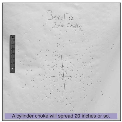
That was zero choke, also called cylinder. The bore of this gun is 0.723 inches and that's about what the choke tube is too, but, of course, there is a little larger-diameter area followed by constriction where the choke tube meets the barrel bore. So call this "cylinder with a choke tube," leaving open the possibility that a fixed – that is, non-choke-tube – cylinder choke might look a little different.
