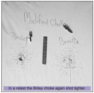
And sure enough, the Briley is making a hole at the center of the pattern at least some of the time, while the Beretta tube does not, producing instead a typical modified "no hole" pattern. As expected, the Briley's pattern is a bit smaller than that of the Beretta in line with its greater shot-concentration in the center.
