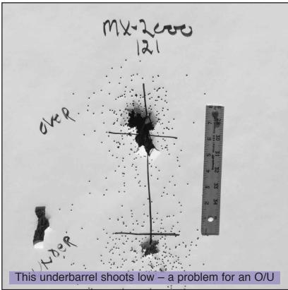
This fault, the lower barrel shooting below the upper by quite a bit, is common enough and such a gun is very difficult to score well at doubles with.
