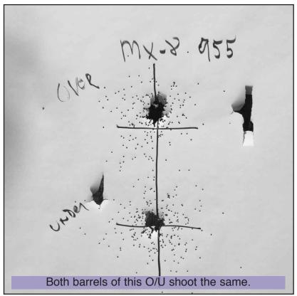
By the way, the lower barrel does not shoot a little lower than the other as it appears to do here. It started lower and has risen more than the upper one has at this distance. This sort of gun just shoots straight, both barrels, and is the holy grail of gun-swappers.
