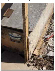
works better than a larger one most of the time. The box should be 12x12 inches of 1/2-inch exterior plywood and be about an inch longer inside than the roll of paper it houses. Leave the front longer so you can bolt some sixfoot uprights on it and secure a crossbar to hang the paper from. Make sure there is a hinged top to keep out the weather. Add a couple of clamps to secure the paper and you are in business.
