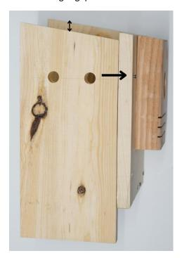
**Step 5:** Nail (D) back panel to (E) right and (F) left panels. Use 3 nails to secure it to the right panel.
