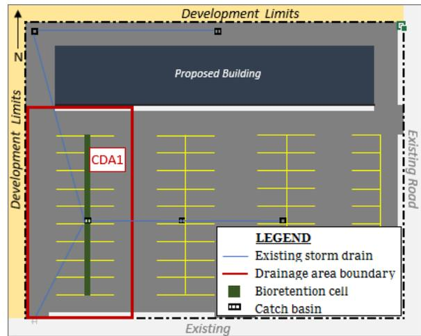
Figure 17: Bioretention cell within the redevelopment's project limits.
