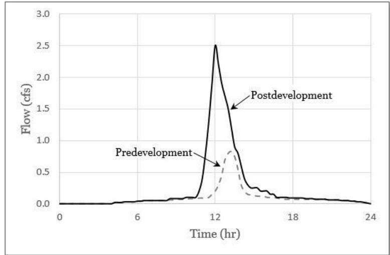
Figure 9: Typical hydrologic impact of development on-site hydrology.
