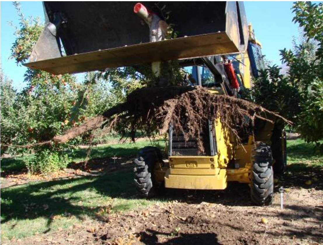
Tractor with hinged-bucket pulled tree trunks from the ground and shook off soil.
