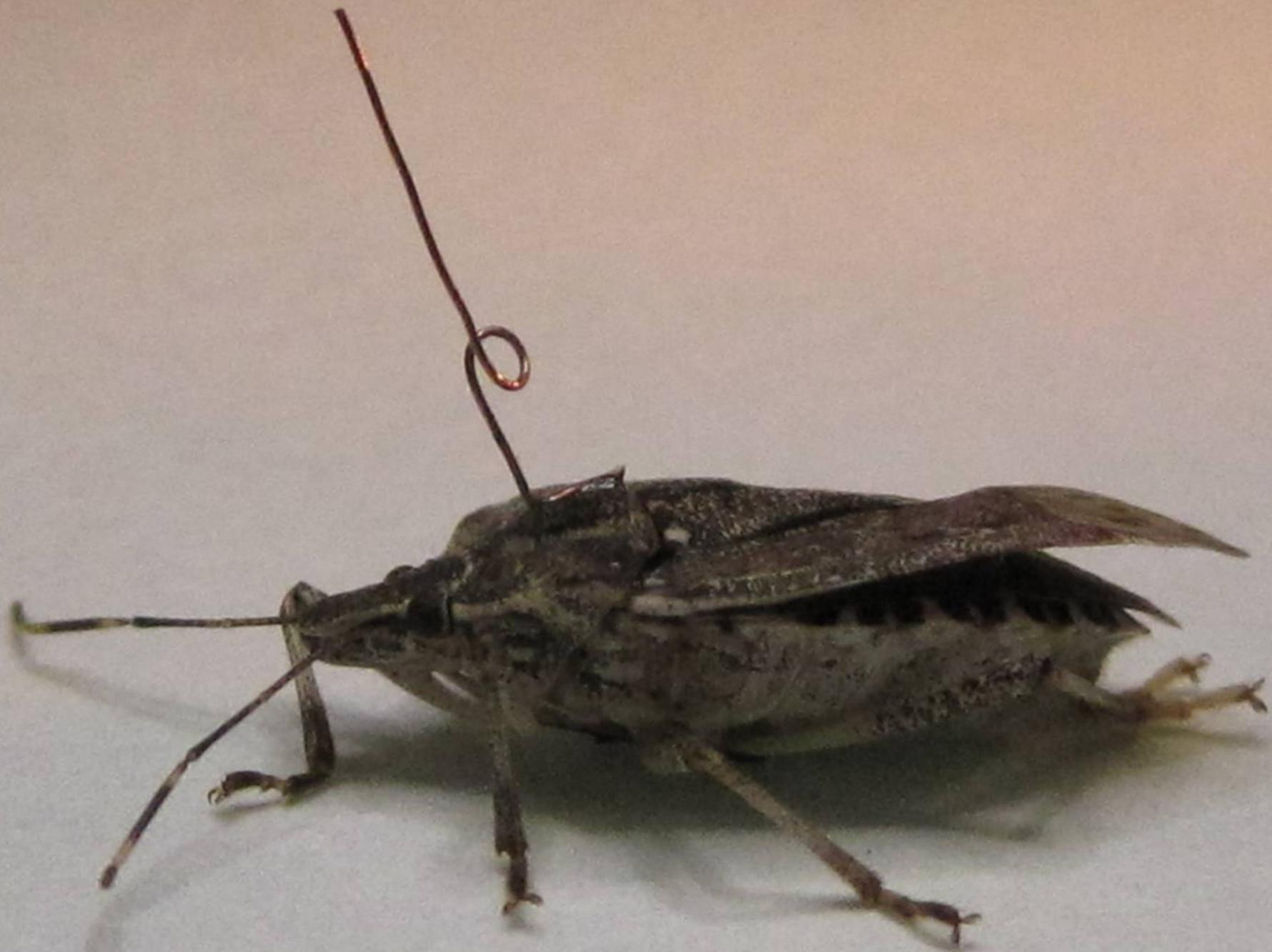
1. Positive detection of the radar-tagged bugs: **100% (n = 30)**
