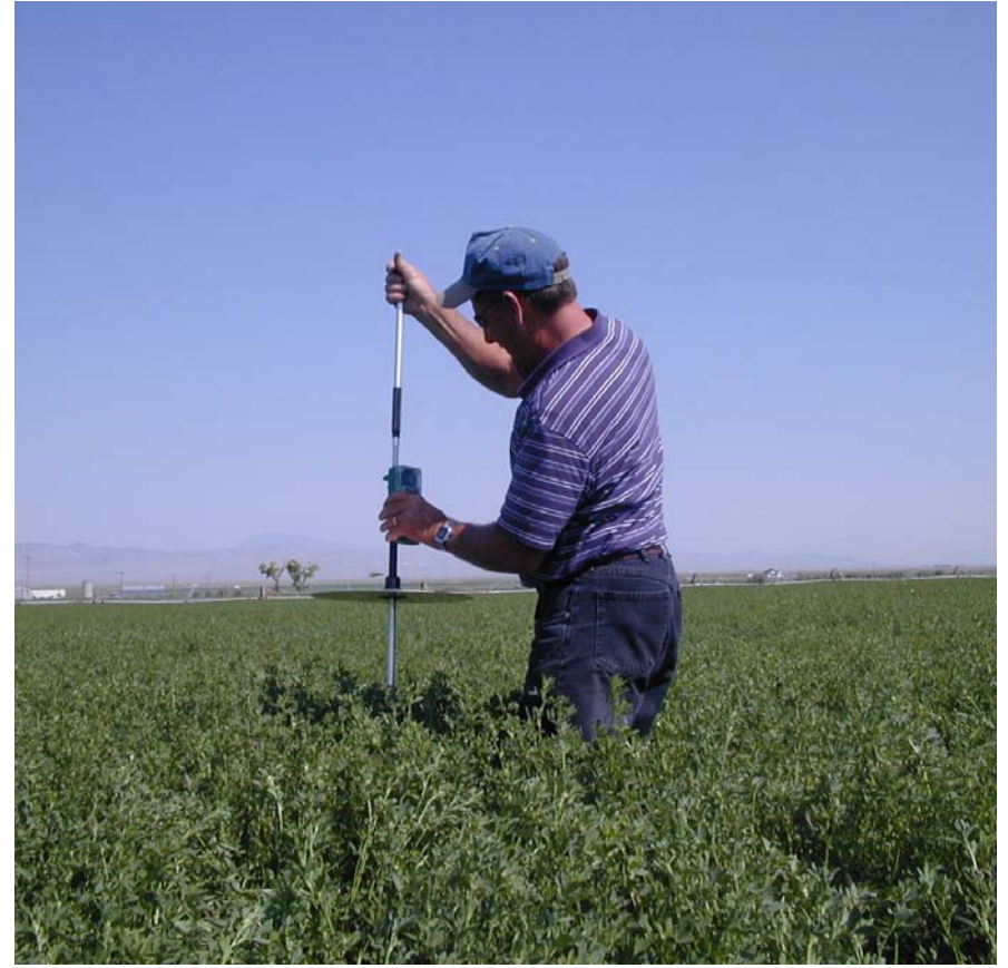
Measuring forage mass with electronic Rising Plate Meter.
