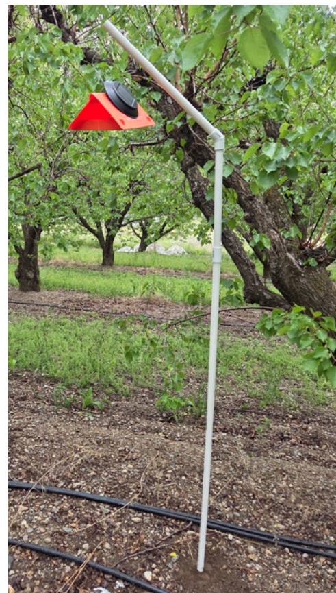
A standard delta trap was modified with the addition of a UV-A light source, and tested with various attractants for peach twig borer.
