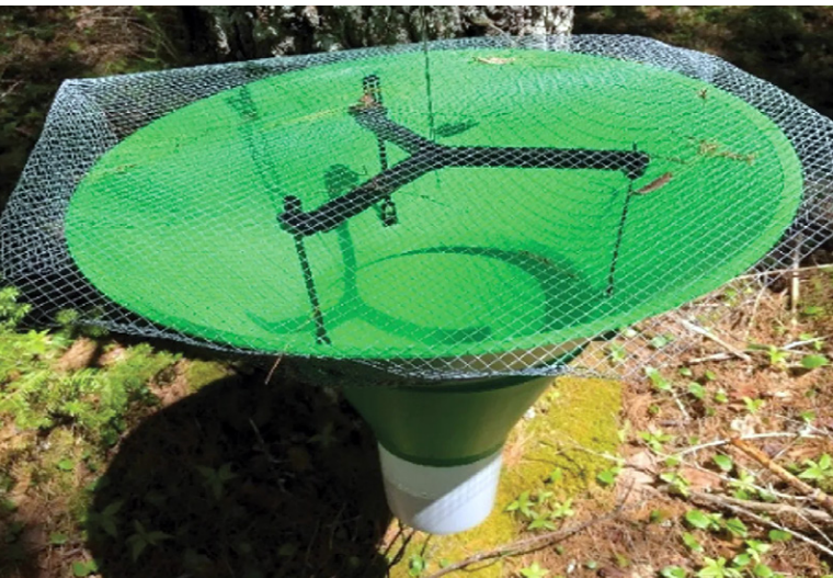
Funnel trap developed by Canadian researchers to detect the hemlock woolly adelgid prior to host symptoms. Image courtesy of Fidgen et al. 2025.
