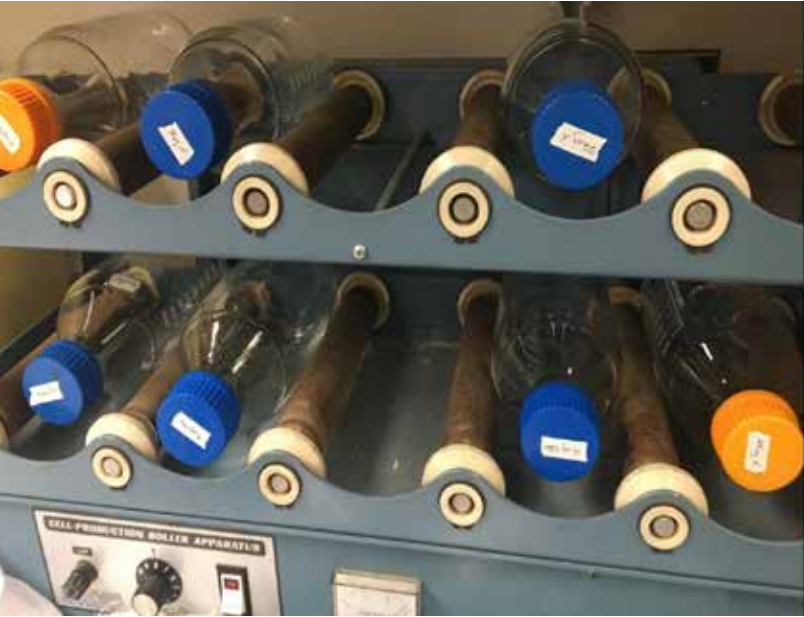
Bottle assays are a way to evaluate the toxicity of contact insecticides. Bottles are first coated with insecticide using a bottle roller (left). Insects are then introduced to the bottle and exposed for 1 hour (right). After 24 hours, the number of insects that die and survive are counted.
