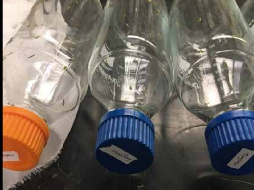
Bottle assays are a way to evaluate the toxicity of contact insecticides. Bottles are first coated with insecticide using a bottle roller (left). Insects are then introduced to the bottle and exposed for 1 hour (right). After 24 hours, the number of insects that die and survive are counted.
