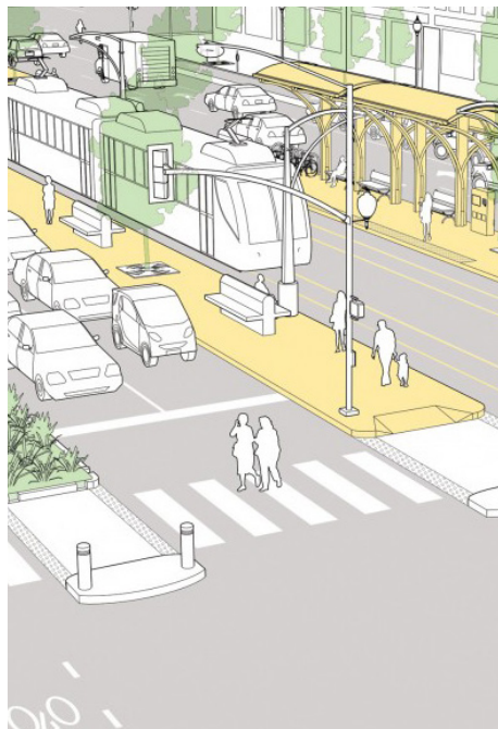
Figure 2.78. NACTO - Transit corridor: NACTO When redesigning streets for high-quality transit service, designers should assess how transit service is impacted not only by the geometry of the corridor, but also its existing signal timing, signal phasing, turns, and other operations that may jeopardize the quality of service.
