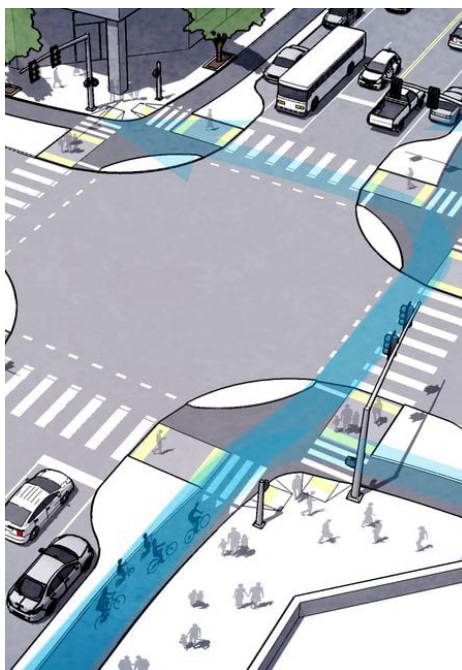
Figure 2.77. Protected bikelanes with bulb-outs and curb extensions, reducing the distance pedestrians and bicyclists have to cross traffic: NACTO
