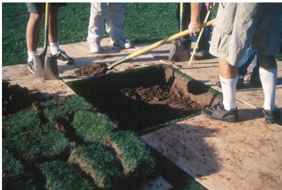
FIGURE 2. EXCAVATION OF LYSIMETER PLOT (SUNBROOK, NOV 2001)
