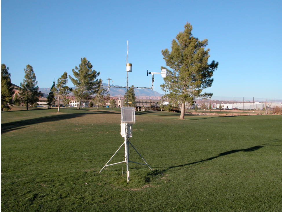
FIGURE 6. TYPICAL ELECTRONIC WEATHER STATION INSTALLATION (SOUTHGATE LOOKING NORTHWARD, 05103 ANEMOMETER)
