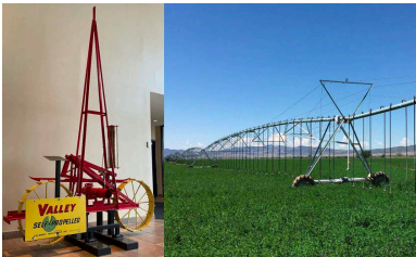
Figure 7. (left) An early Valley center pivot on display at the Valmont Industries Headquarters, Valley, NE; (right) A modern center pivot.
