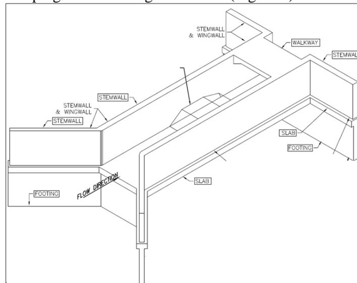
Figure 2. TCID's standard design for Replogle flumes
