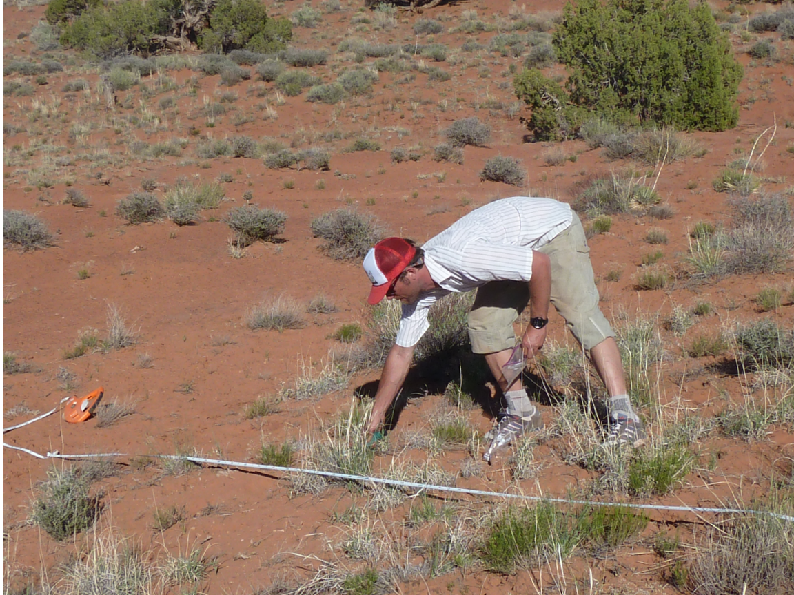
Figure 15. Field technician conducting a line-point intercept in lower Indian Creek, UT.
