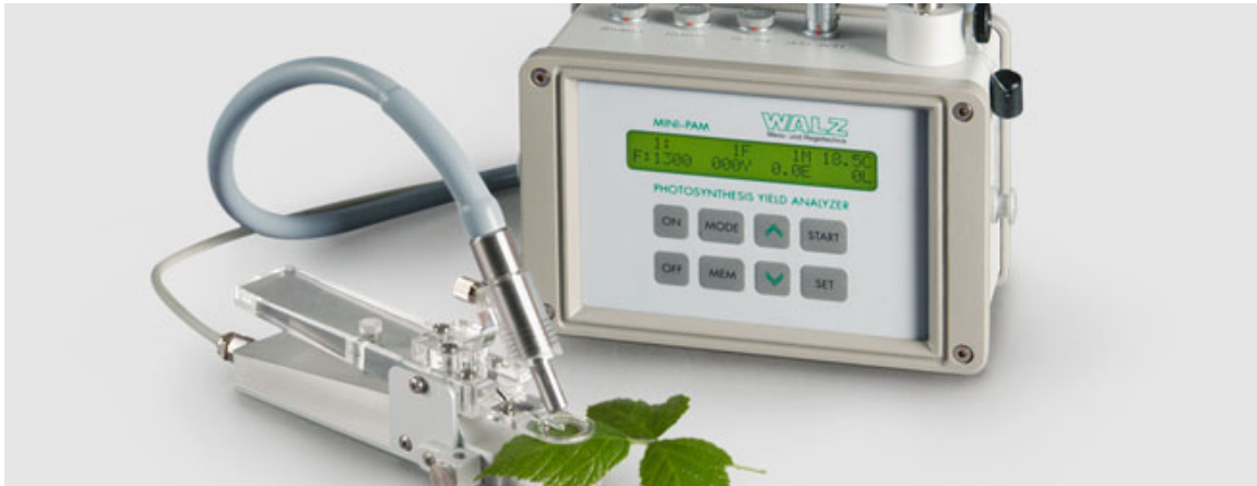
Figure 28. Walz™ Mini-PAM Photosynthesis Yield Analyzer.
