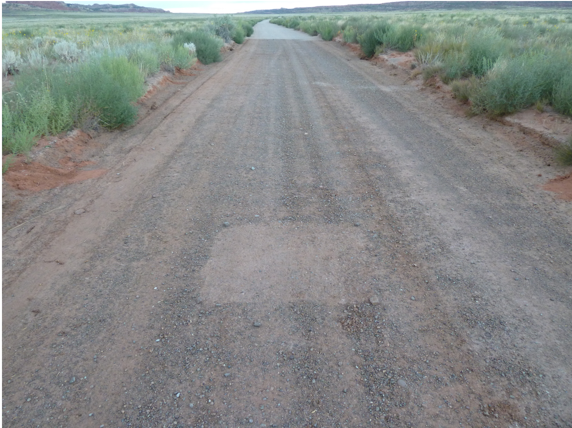
Figure 24. 1\text{ m}^2 quad that has been sampled for road sediment
