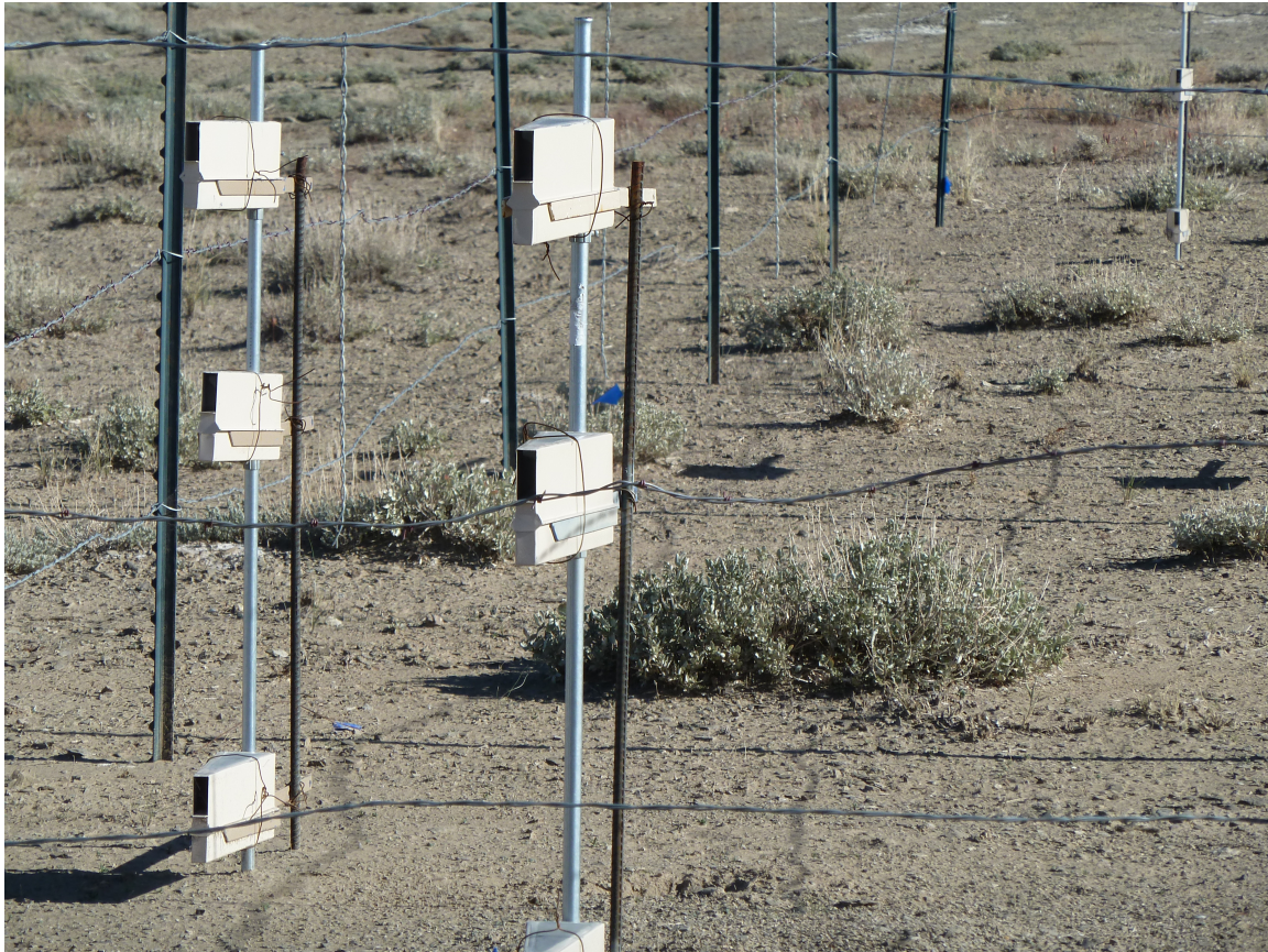
Figure 23. BSNE units fixed in place using rebar and bailing wire to prevent rotation in shifting winds.
