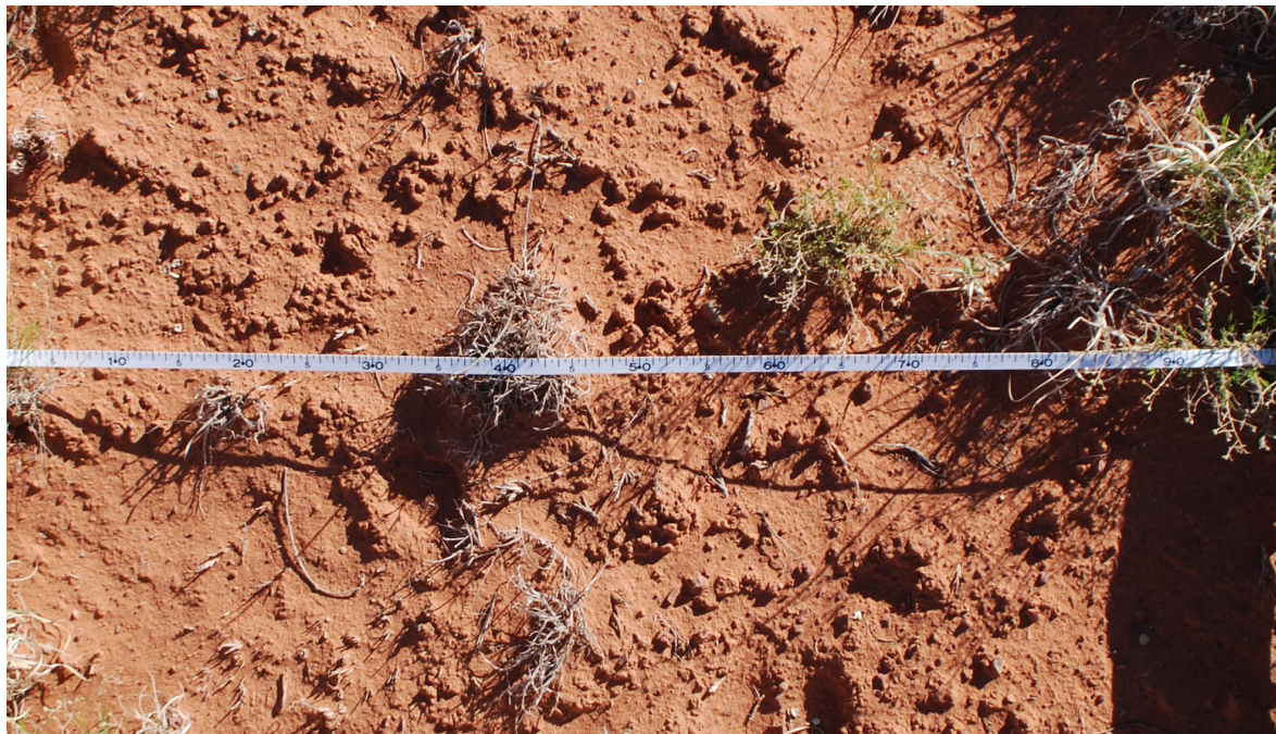
Figure 19. Transect in place for gap distance measurement.
