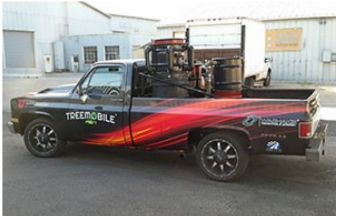
Eddings and Whitty's Treemobile, powered by gasification of wood pellets; see it out on the road at treemobile.chemeng.utah.edu
