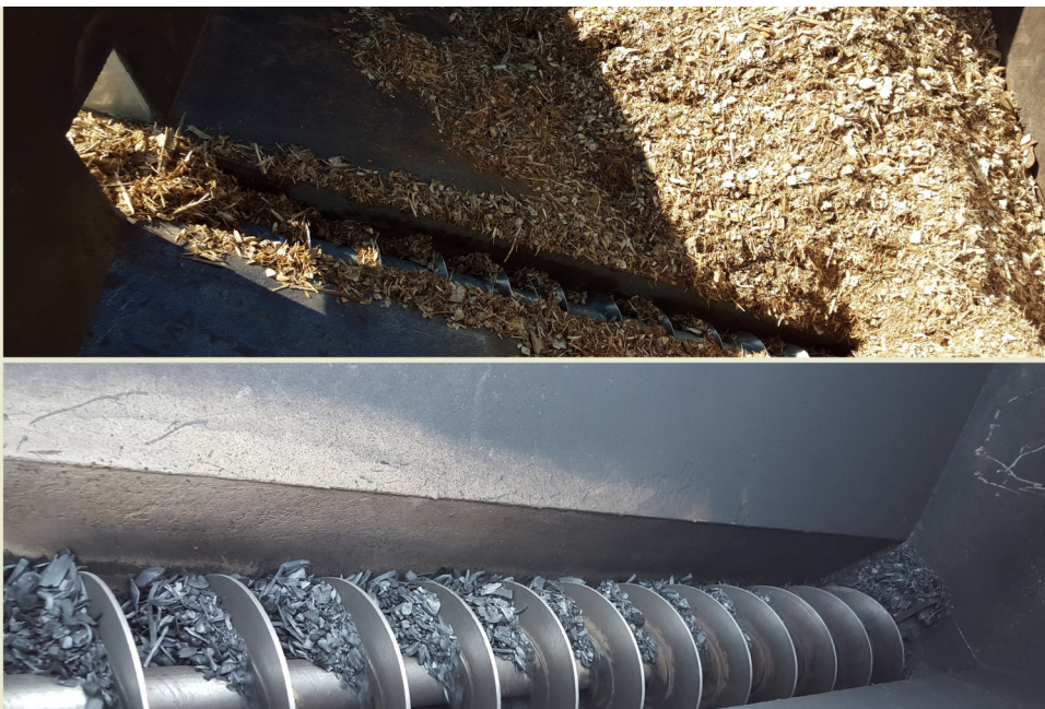
Feedstock being fed into the mobile pyrolysis unit (top); finished product, biochar following pyrolysis (bottom).
