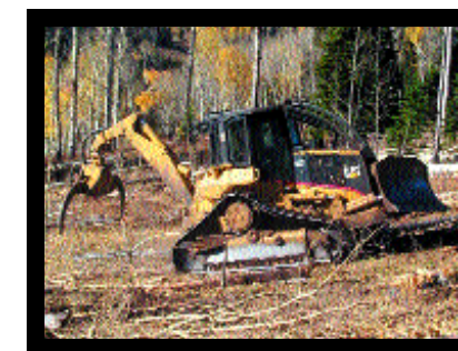
Tracked grapple dozer: Suitable for use on moderate slopes. May cause less damage than rubber tired skidders when soils are wet.
