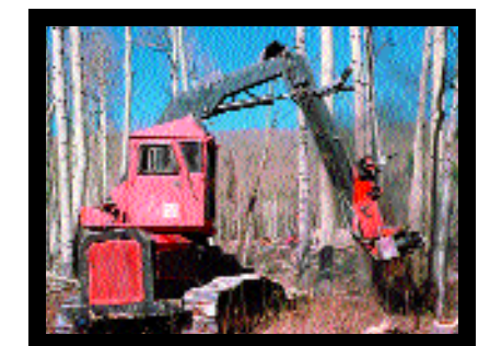
Feller-buncher: Mechanical harvesters can minimize damage to residual trees, water & soil.
