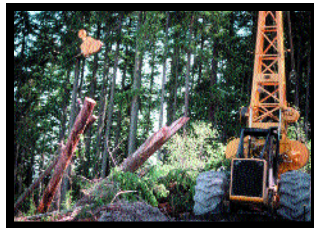
Cable harvesting system using a tower and drum assembly.
