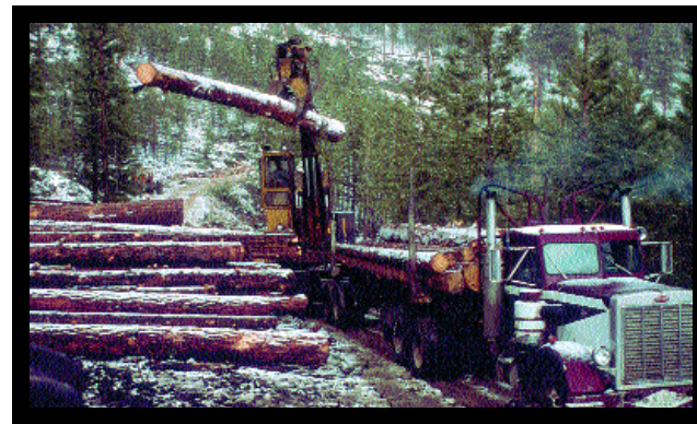
Decking logs along a road is one way to minimize the number of landings needed
