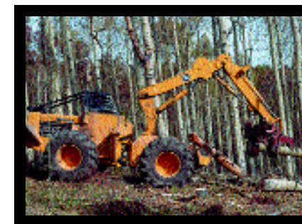
Rubber tired grapple skidder: The most commonly used and least expensive system. Skidders may cause excessive soil damage (i.e. compaction) if operating in wet conditions.
