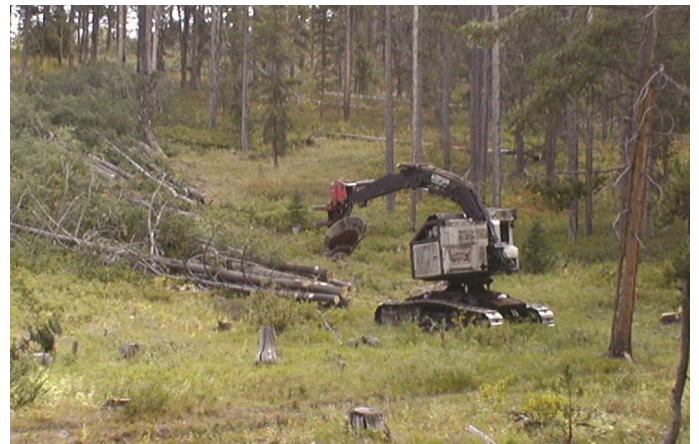
Use of a feller-buncher and directional felling can help minimize soil disturbance in the SMZ.
