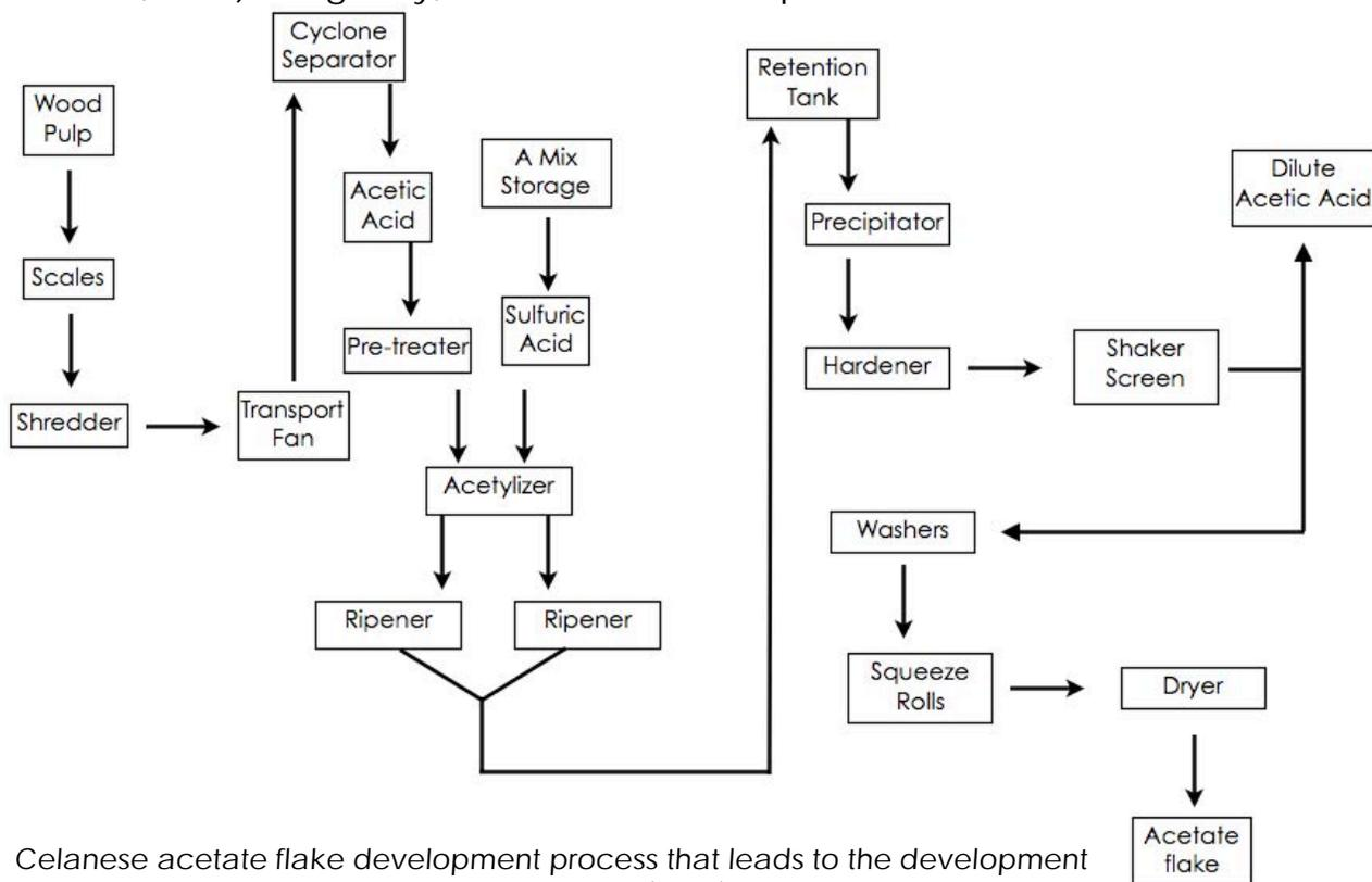
Figure 1: Celanese acetate flake development process that leads to the development of acetate fabric adapted from Celanese Corporation (2012).
