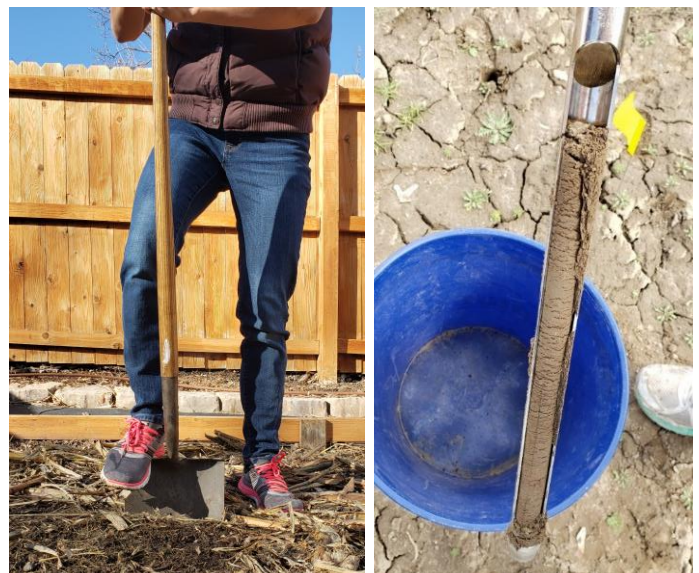
Figure 4. Collecting soil samples for soil testing with a shovel (left) or soil corer (right).
