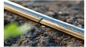
The Dripline (20) consists of built-in precision emitters every 4" of 0.134 gallon per hour (0.40 gph/ft of length)
