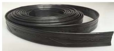
The Dripline (20) consists of built-in precision emitters every 4" of 0.134 gallon per hour (0.40 gph/ft of length)
