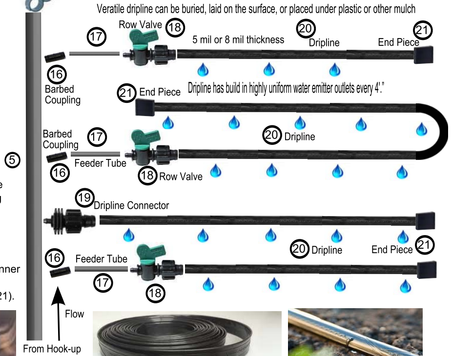
The Dripline (20) consists of built-in precision emitters every 4" of 0.134 gallon per hour (0.40 gph/ft of length)
