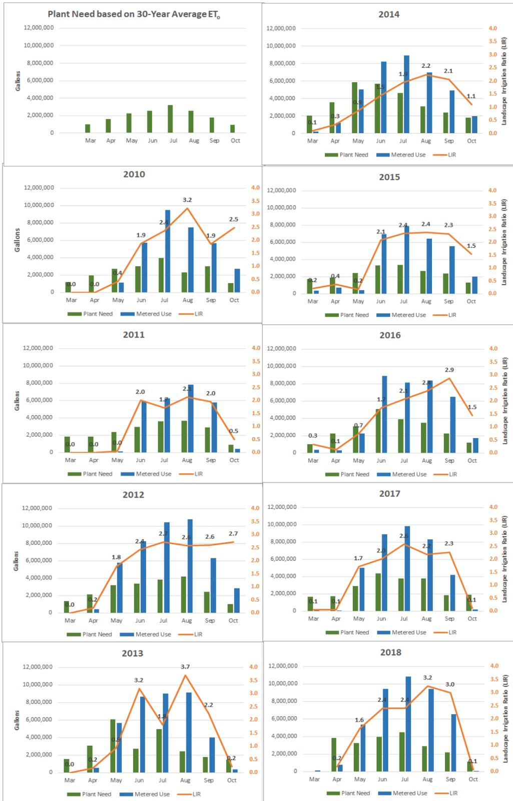
**Figure 9. WaterMAPS™ monthly analysis for Utah State Capitol by year (2010 – 2018) with reference to 30-year average (1979-2008) ET<sub>o</sub>-based plant water need. Each annual panel shows plant water need (green bars) compared to metered water use (blue bars) with LIRs (orange lines and numbers).**
