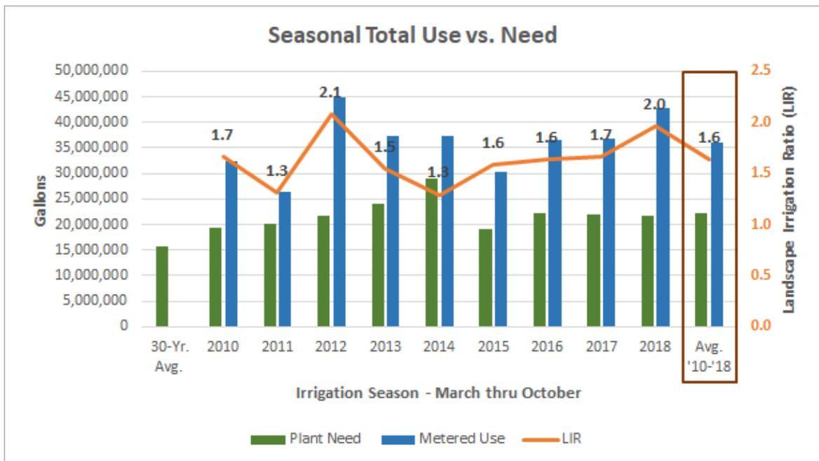
**Figure 8. WaterMAPS™ annual analysis, 2010-2018, for Utah State Capitol with the nine-year average in red box. Plant water need (green bars) is compared to metered water use (blue bars) and the calculated LIR for each year is displayed in numbers above orange bar. Plant water need of the Capitol grounds based on the 30-year average (1979-2008)  $ET_o$  is shown in the left-hand column.**
