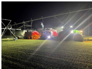
Figure 1. The Baler Used for All Experiment Treatments Was Outfitted With a Staheli West DewPoint Steamer (left) and a Harvest Tec Dew Simulator (right)
