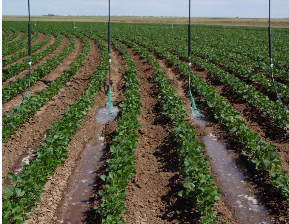
Figure 50. LEPA on a row crop using drag socks to minimize erosion to the furrow dikes that limit water movement in the furrows.
