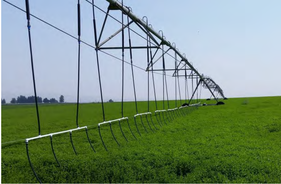
Figure 51. LEPA on mint. This setup allows conversion back to MESA for better crop germination if desired.
