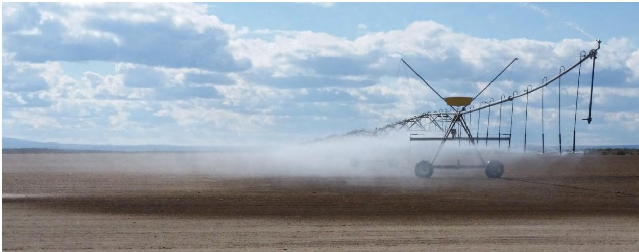
Figure 32. Water being lost to the wind on a center-pivot irrigation system. Only the droplets are visible. Water losses once converted to water vapor are no longer visible.
