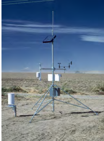
Figure 37. An automatic weather measurement station in agricultural conditions.
