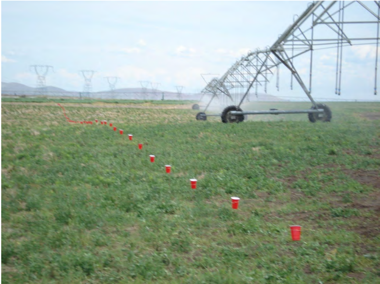
Figure 25. A uniformity evaluation of a center pivot using catch cans.
