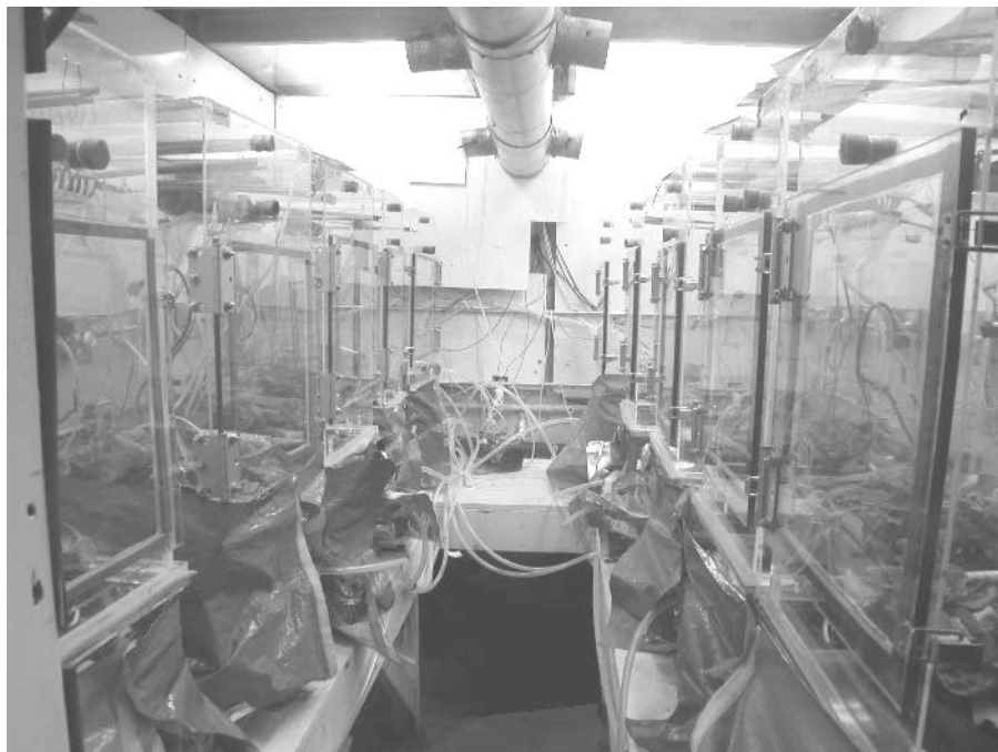
Fig. 1. The 10-chamber gas-exchange system used in Study 1. There are five chambers on each side of a walk-in growth chamber. Each chamber has a reflective skirt wrapped around the outside to minimize side lighting.
