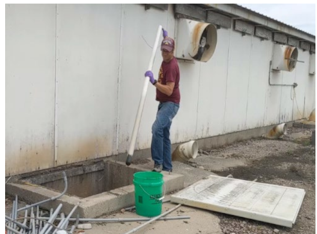
Figure 12. Slurry Sample Collection Using Column Sampler and Access Port
