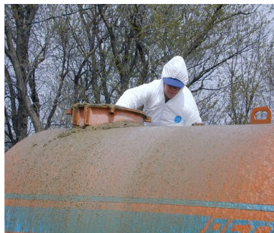
Figure 10. Sampling Liquid Manure From Tank During Pump-Out
