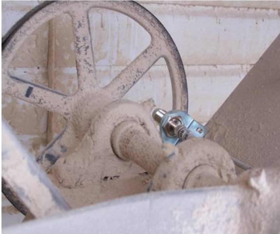
Figure 10. Location of induction sensor on fan motor.
