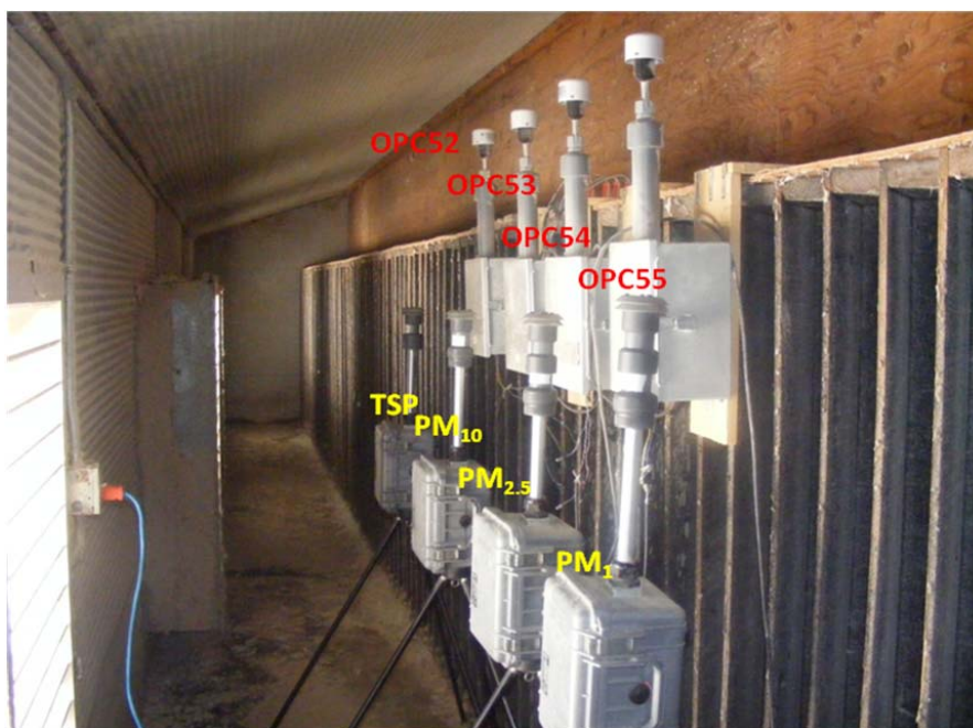
Figure 14. Array of OPCs and MiniVols in the poultry building.
