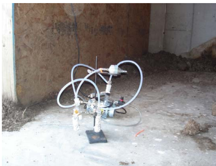
Figure 17. Impinger sampling train at north door of the manure barn on October 6 th , 2008.
