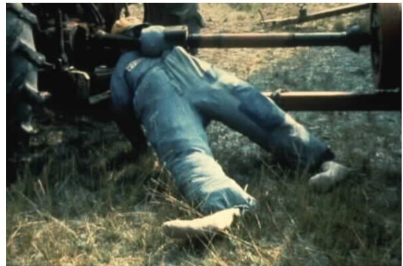
Figure 1. Coveralls stuffed with straw demonstrates the power of a rotating PTO shaft catching loose clothing (BHHHC). 4
