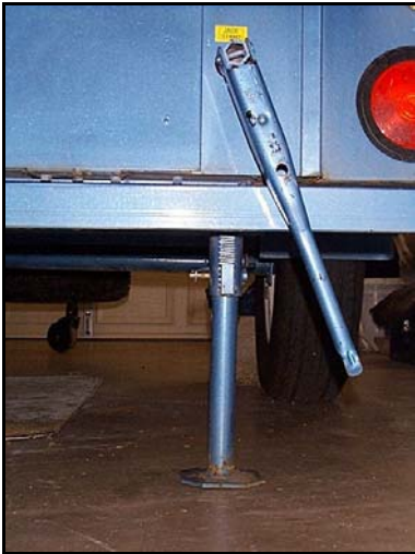
Jacks at rear of trailer are used to level side-to-side. They can also be used to replace a tire.
