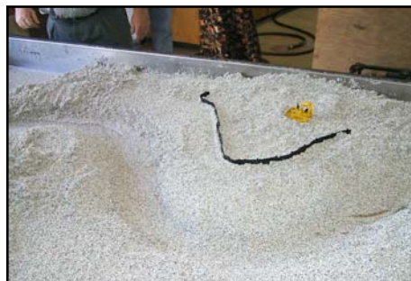
Installation of silt fence.
