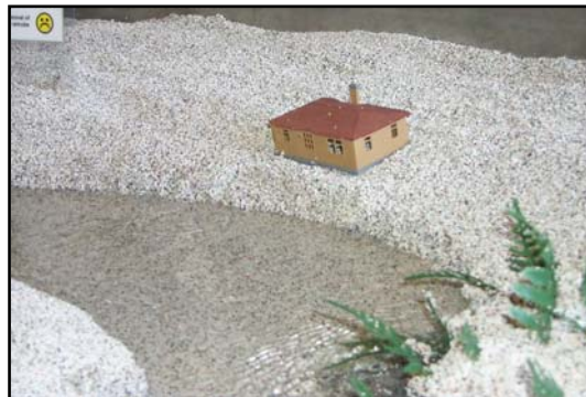
Set one house to fall in the river when bank cutting occurs.
