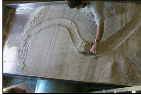
Dig out the channel with scoop.
