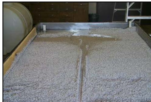
Dig out a reservoir at top of slope connecting inlet to starting point of channel. Cut a shallow, straight groove down center.
