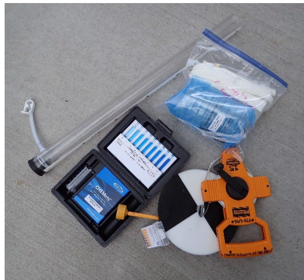
Tier 1 monitoring equipment - thermometer, pH strips, dissolved oxygen kit, turbidity tube or Secchi disk, and E. coli testing supplies.
