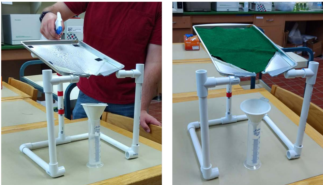
Figure 7. Urban and natural watershed PVC stand setup. Note the Velcro on the urban setup to attach felt pieces. See the setup instructions on the next page.
