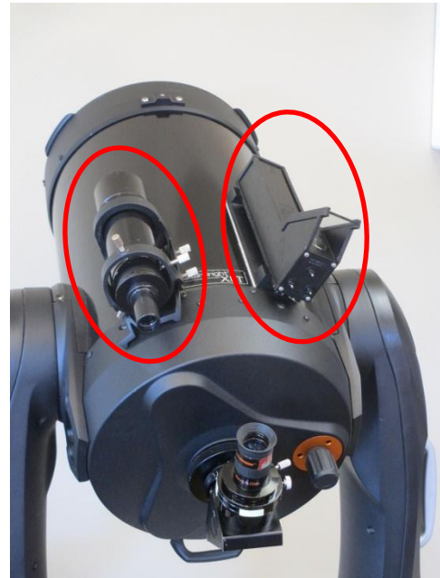
Figure 15-A Schmidt-Cassegrain telescope equipped with a traditional finder telescope (left) and a Telrad zero-power finder (right). (NPS /Zach Schierl)
