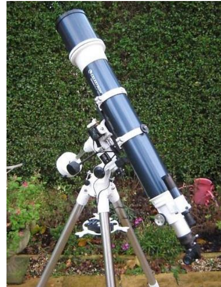
Figure 5-A 120mm backyard refracting telescope. The eyepiece is located at bottom right. (Wikimedia user: fractal.scatter, public domain)
