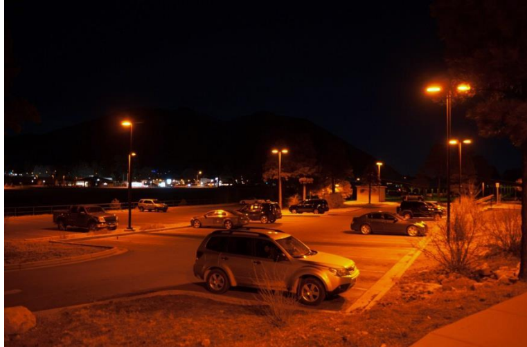
Figure 10-A parking lot in Flagstaff, AZ illuminated by low-pressure sodium lamps with a color temperature of ~1800K. (Zach Schierl)
