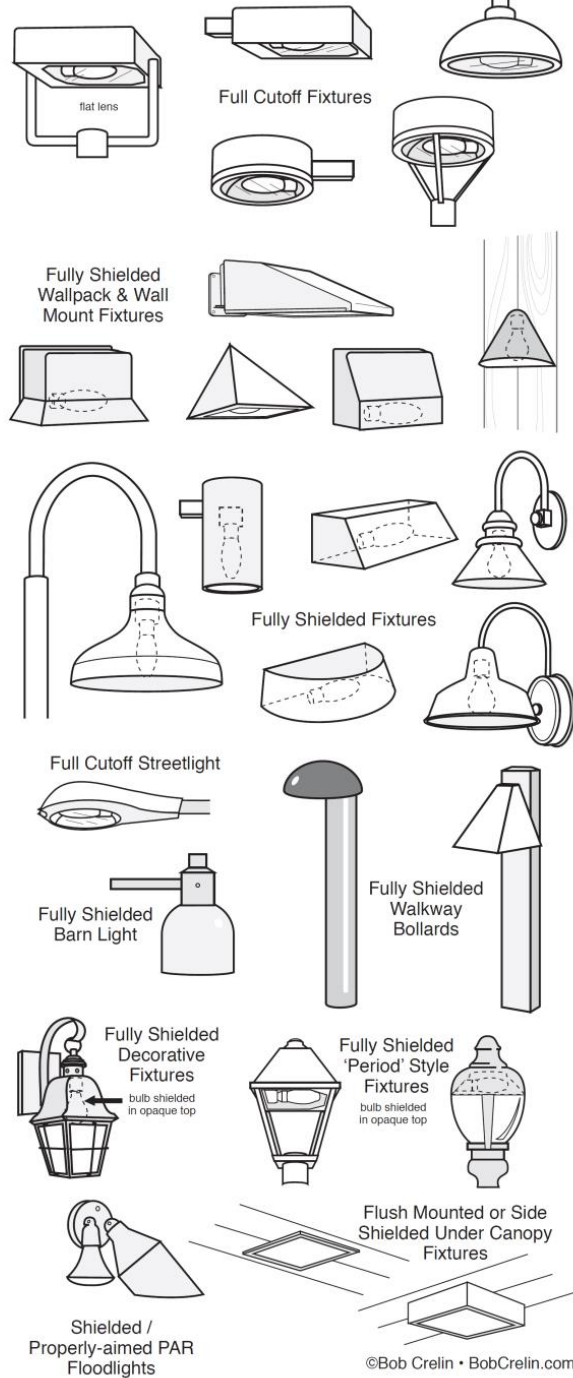
Figure 5-Examples of poorly designed light fixtures (left column) and dark-sky friendly light fixtures (right column). Note that many newer LED fixtures behave differently with regards to glare and light trespass, and are not depicted here. (Robert Crelin)
