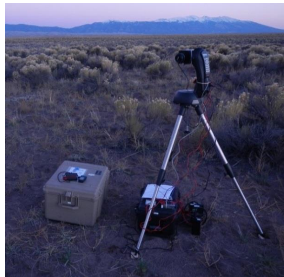
Figure 9-NPS CCD camera setup for measuring sky luminance. (Natural Sounds & Night Skies Division/NPS)
