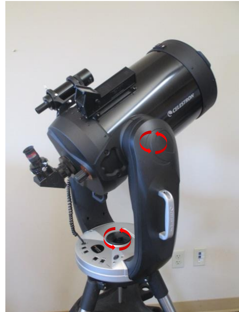
Figure 8-A Schmidt-Cassegrain telescope on an altazimuth mount. Red arrows indicate the axes of rotation. (NPS/Zach Schierl)
