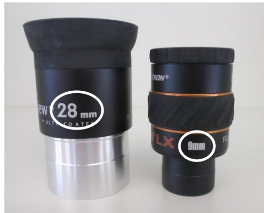
Figure 5-The two standard eyepiece barrel sizes: 2" (left) and 1.25" (right). The 28mm eyepiece will provide a low magnification view, which the 9mm eyepiece will provide a higher magnification view. (NPS/Zach Schierl)
