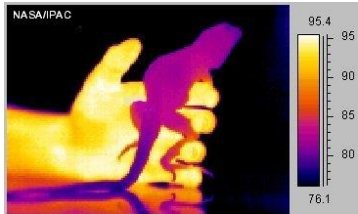
Figure 2-Infrared image of a lizard in a human hand. This is a false color image, meaning that the colors are not true, but used to represent varying intensities of infrared radiation, which would otherwise be invisible to the human eye. (NASA/IPAC/Caltech)
