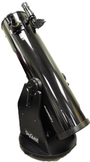
Figure 9-A 10" reflecting telescope on a Dobsonian mount. (NPS/Zach Schierl)
