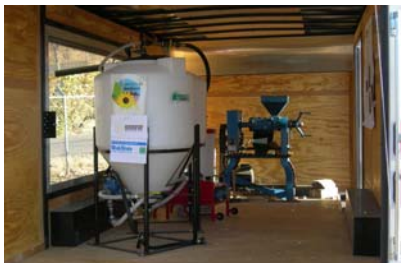
Figure 1. Mobile (trailer mounted) research and demonstration biodiesel processor and oil seed press. This equipment is currently available to farmers for on-farm fuel production. Funds were provided by UDAF and NRCS.
