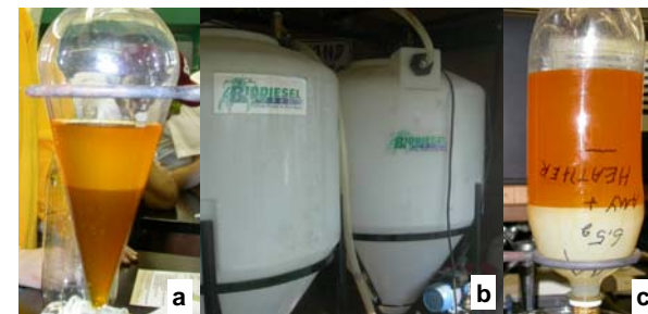
Figure 5a,b,&c. a. An example of biodiesel on top and glycerin below in a separatory funnel; b, the reaction tank (left) and the washing tank (right) of the biodiesel processor; c, washed biodiesel on top and wash water below in a plastic bottle.
