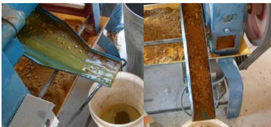
Figure 2. Oil seed screw press separating oil (left) and seed meal or cake (right) from camelina seed. Press is belt driven by a 5hp 220v motor.
