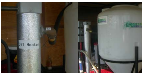
Figure 3. Two pictures of the biodiesel processor with the first reaction tank and electric recirculating oil heater
