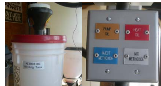
Figure 4. Methoxide mixing tank (left) where methanol and lye are combined before injecting into hot oil. Biodiesel processor control panel (right).
