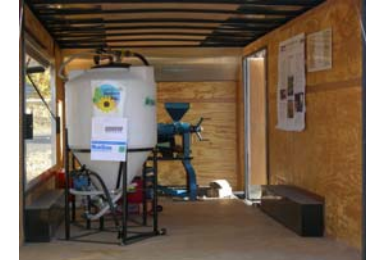
Figure 5. Central Utah Biodiesel Project mobile oil-seed and biodiesel research and demonstration processing trailer. Biodiesel reactor in the foreground and screw-type oilseed press (back).
