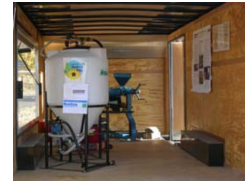
Figure 5. Central Utah Biodiesel Project mobile oil-seed and biodiesel research and demonstration processing trailer. Biodiesel reactor in the foreground and screw-type oilseed press (back).
