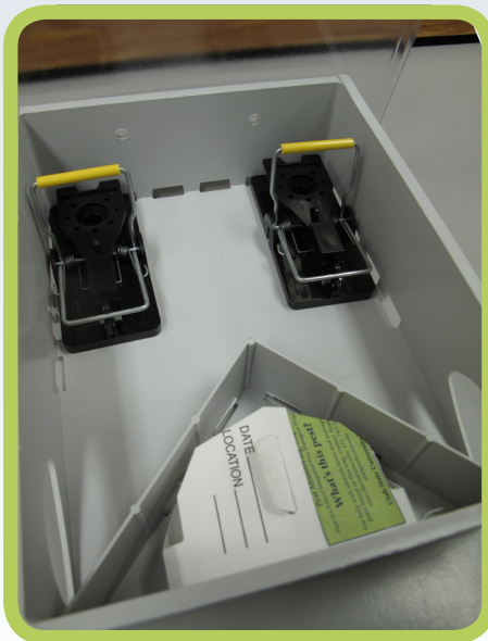
Right: Figure 2. Dual-purpose mouse and arthropod monitoring/trapping station.
