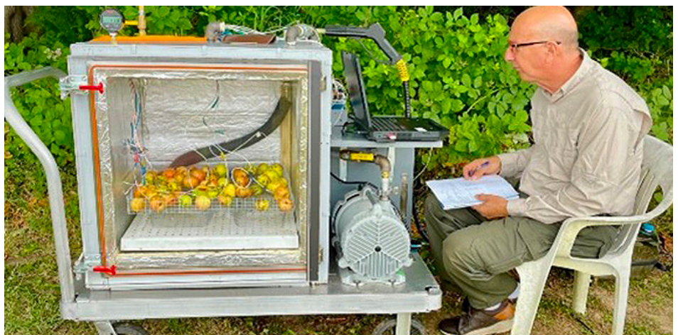
Biological Science Laboratory Technician Luis Bradshaw conducts apple maggot treatment trials using the stainless-steel vacuum steam prototype. USDA AHPIS
