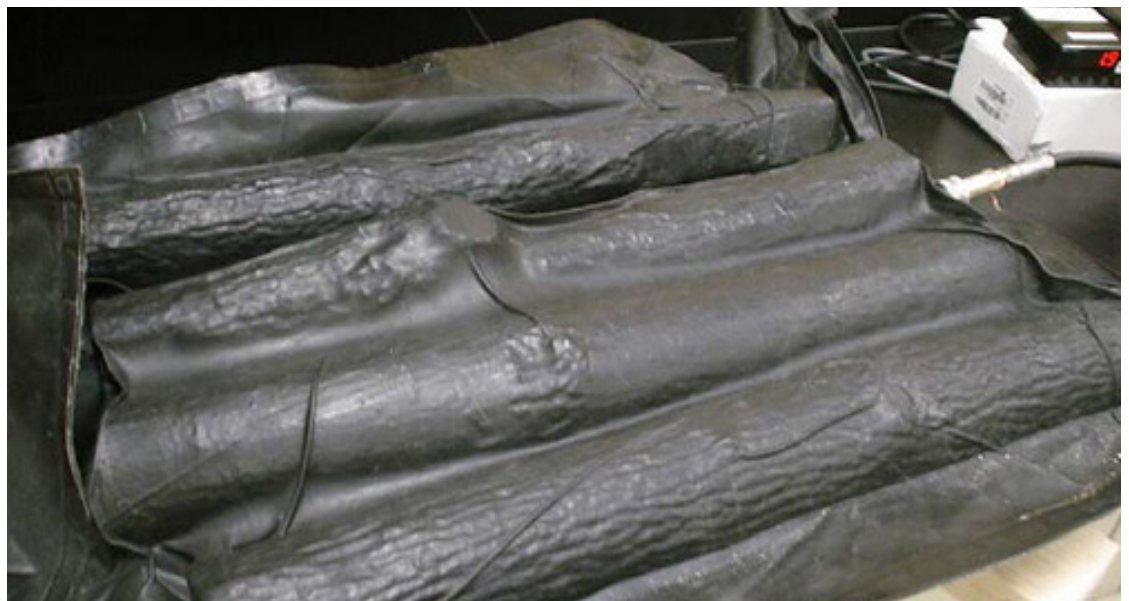
Ash logs undergoing vacuum treatment to kill emerald ash borer larvae. U.S. Forest Service
