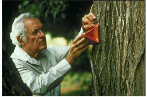
Delta paper trap used by survey personnel for detecting adult gypsy moth. The traps are baited with the female pheromone which attracts the male moth. The sticky surfaces inside the trap catches moths. USDA APHIS PPQ, USDA APHIS PPQ, Bugwood.org
