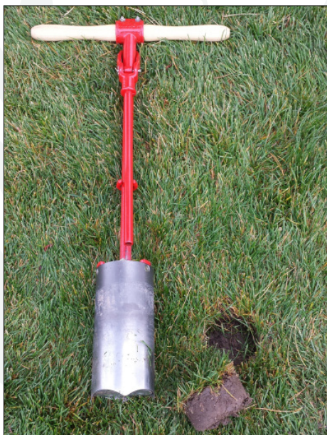
Fig 17. A soil corer can be used to collect soil and root samples.
