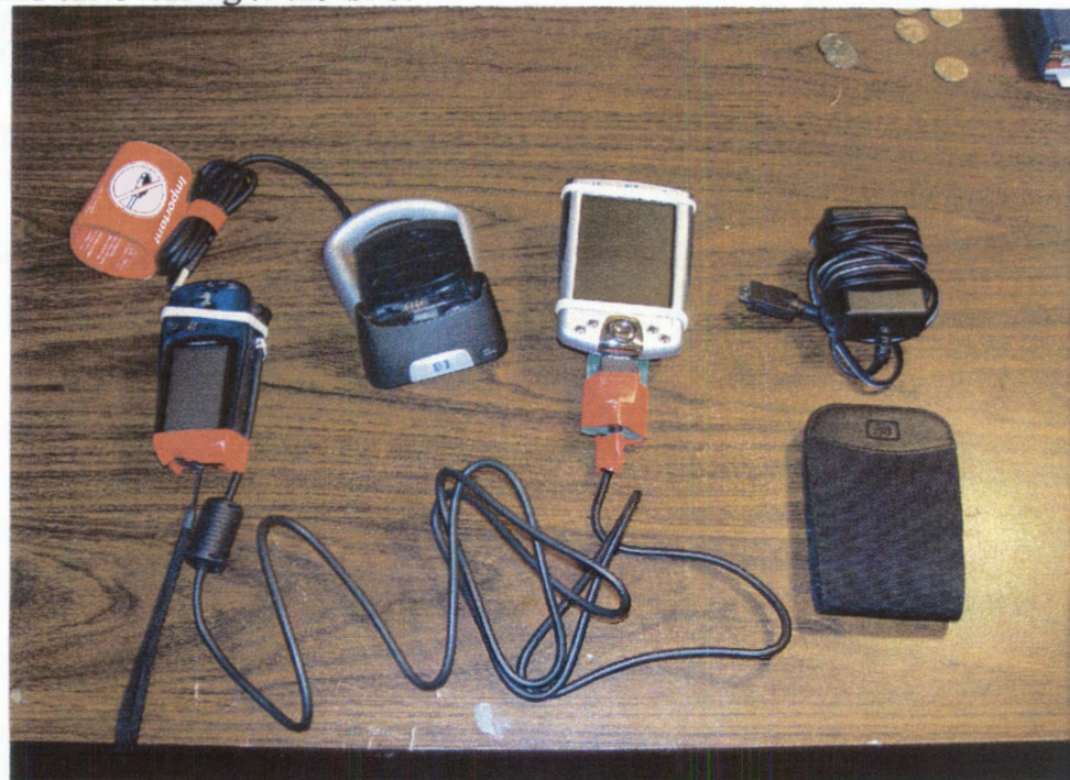
The cradle consists of a length of plastic ruler to which the data cable is taped with red tape. The iPAQ simply plugs in and is attached with the two rubber bands as in the picture
