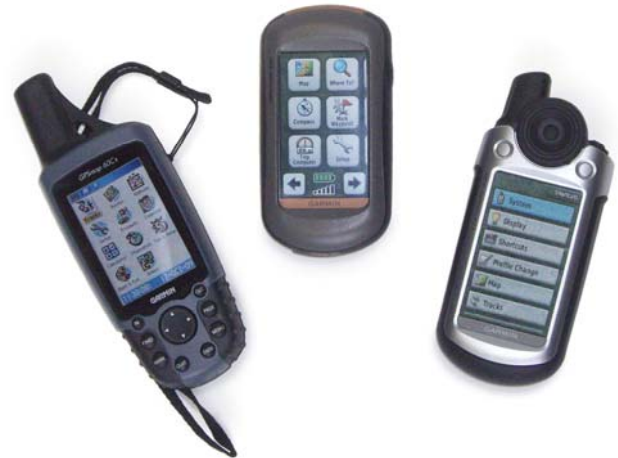
These three Garmin handheld units each use different high-sensitivity GPS chipsets. From left to right, the GPSmap 60Cx, Oregon 300, and Colorado 400t. These units are superior to earlier models in TTFF (time to first fix) and in tracking under tree canopy.
