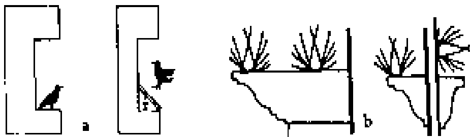
Figure 2. Wooden, metal or plexiglass covering over a ledge at a 45° (a) or porcupine wires (b) can be used to prevent roosting and nesting.
