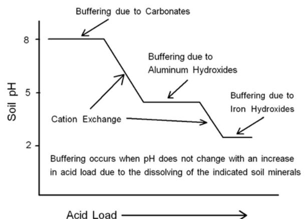
Figure 1. pH buffering effects in Utah soils.
