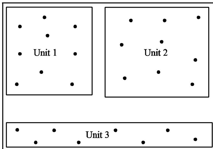
**Figure 1.** Soil sampling patterns for three separate units in an area. Each dot represents one sample. Individual samples within a unit should be combined to make the composite sample. Units may be separate farm fields or different areas in the landscape.
