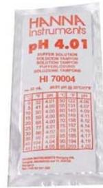
Calibration is often specific to each meter. Typically, the electrode is placed into pH 4.01 and the reading is taken. A manual of automatic system is used to adjust the reading to pH 4.01. This is followed rinsing the electrode and placing the electrode into pH 7.0 buffer and adjusting the reading to 7.0.
